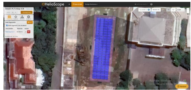
Fig. 8. Solar Panel Placement
