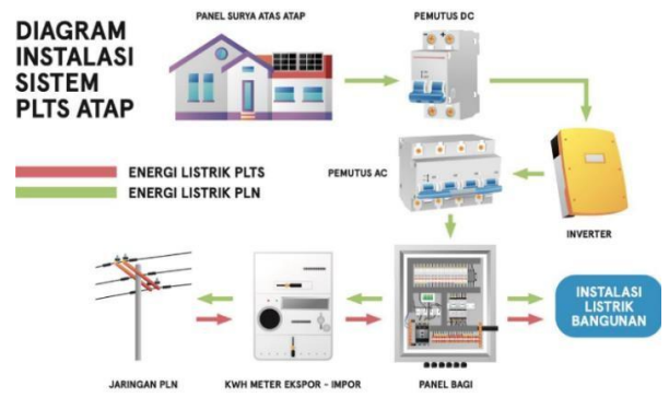
Fig. 1. Diagram of On-Grid Rooftop Solar System
